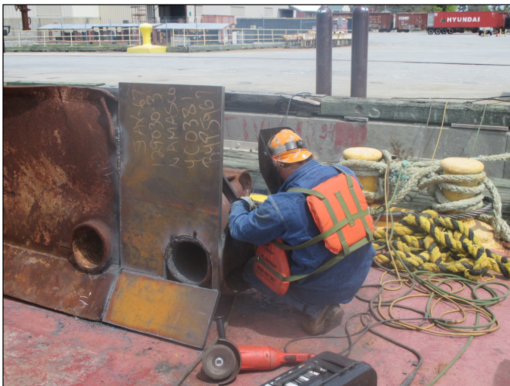
Figure 3. GLDD personnel welding metal extensions to bed leveler blade face.
